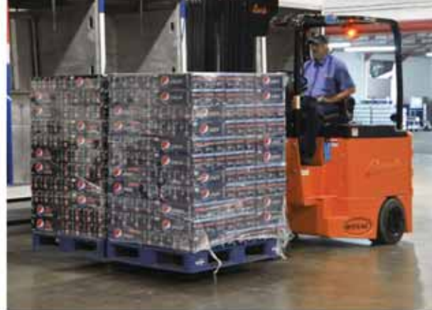
● Handle two pallets at a time ● Full Cold Store Cab -30
